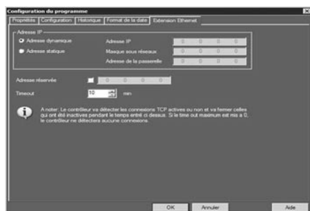
Ethernet communication module configuration window
